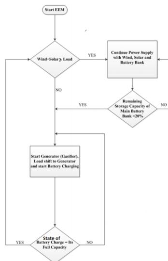
Figure 6: Decision matrix in control module for implementation of source hierarchy during start-up. This matrix ensures that the load demand is met, use of renewable sources is maximized, and the charge of the battery bank does not fall below 20%
