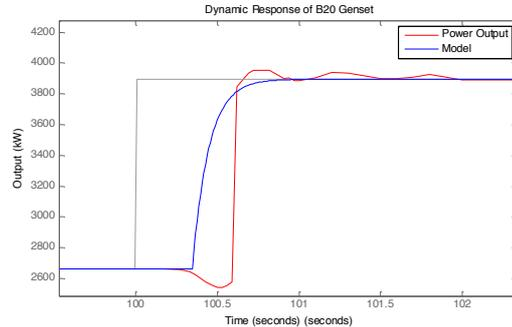
Figure 12: A zoomed in view of the experimental results and model response to a load increase
