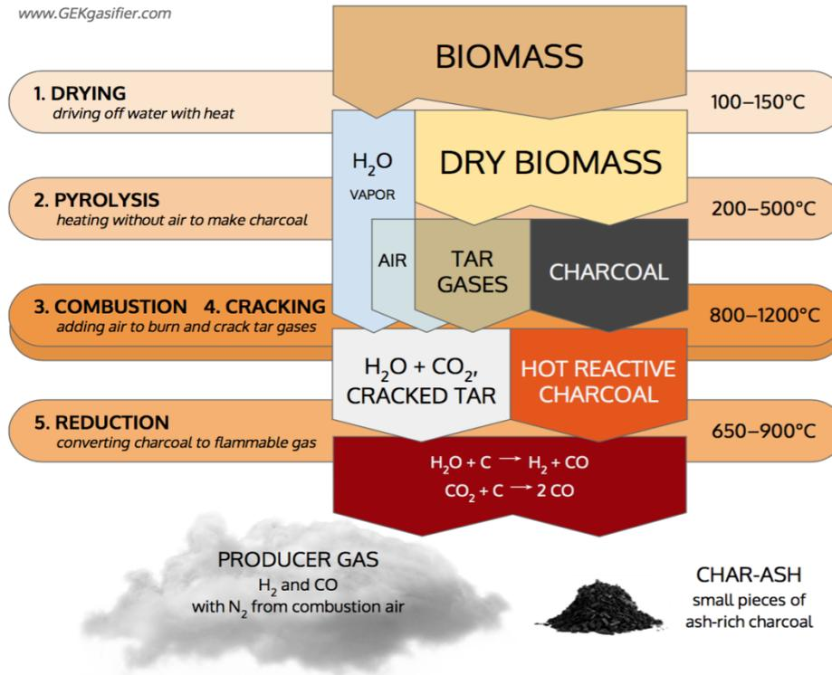
Figure 2: Summary of the characteristics of the main processes of gasification
