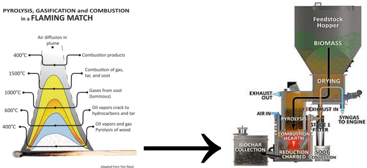
Figure 1: While complete combustion Gasifiers, shown on right, separate discrete thermal processes by controlling air intake and temperatures that otherwise
