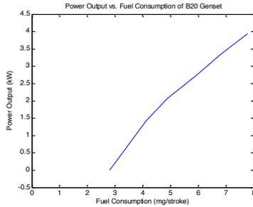
Figure 8: Power Output vs. Fuel Consumption of B20 Genset
