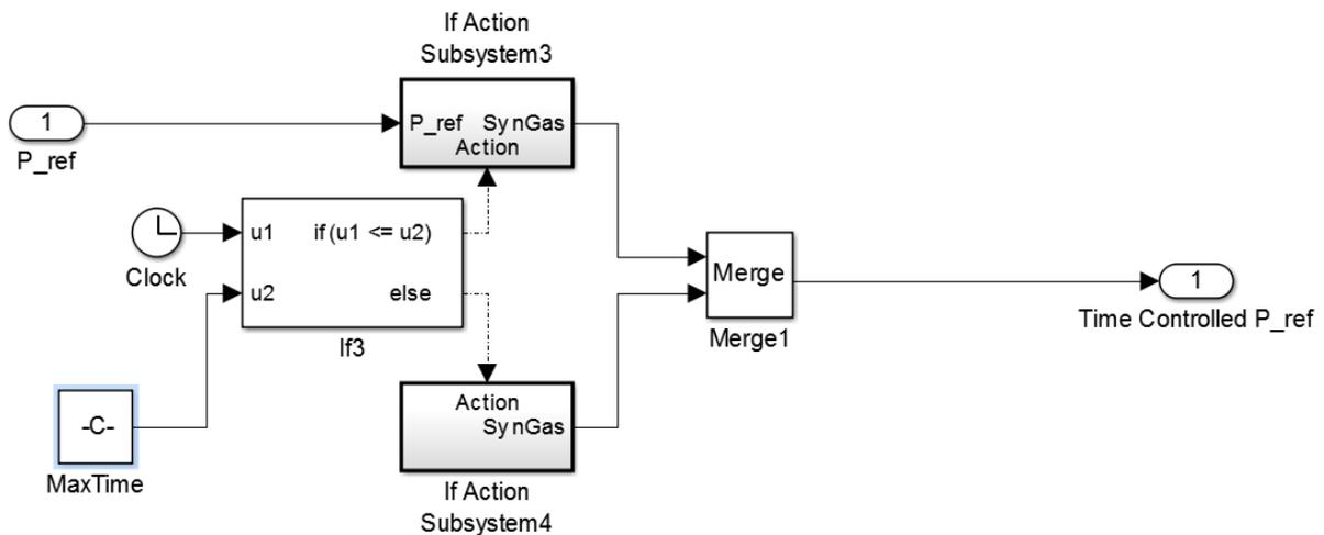
Figure 14: Maximum Time Length of Operation Control Subsystem. MaxTime is set to 43200 seconds, or 12 hours
